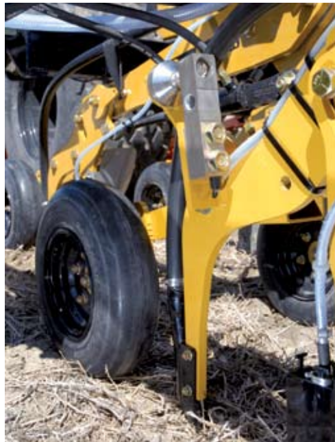
The new Packing Force Sensor Mounts just above the packer wheel. It measures changes in packing pressure, allowing farmers to make accurate adjustments for uniform packing.
