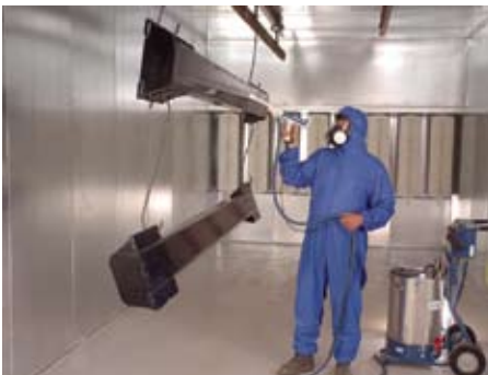
Straw Track Finishing Supervisor, Leonard Wollbaum, applies powder coat paint to Seed Master components.
