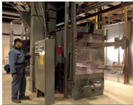
Steel beams enter the blasting chamber for cleaning.
